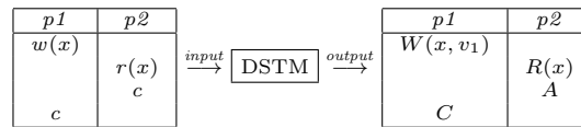
Fig. 3. A simple input pattern for which DSTM produces a commit-abort ratio of \tau = 0.5 (transaction of p2 aborts).
